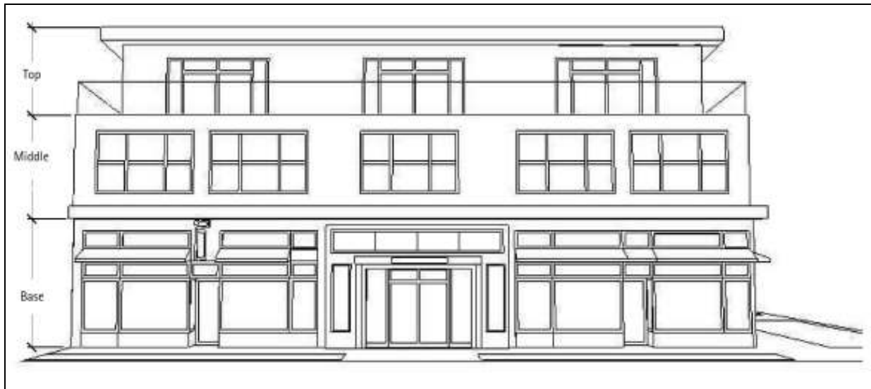
Articulated building with clearly defined base, middle and top.
