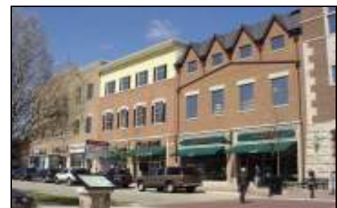
Facades should be “broken up” with articulation and roofline changes to create a “built over time” appearance.
