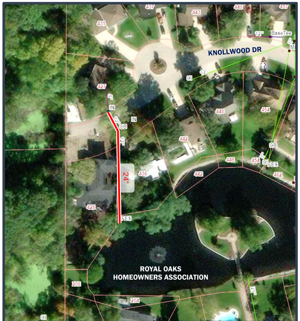
FIGURE 14: Proposed storm sewer improvements in Area 3 from Knollwood Dr to Royal Oaks Homeowners Association Pond
