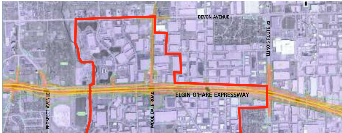
Figure 3.2: Preliminary IDOT Alignment for Elgin O'Hare Expressway
