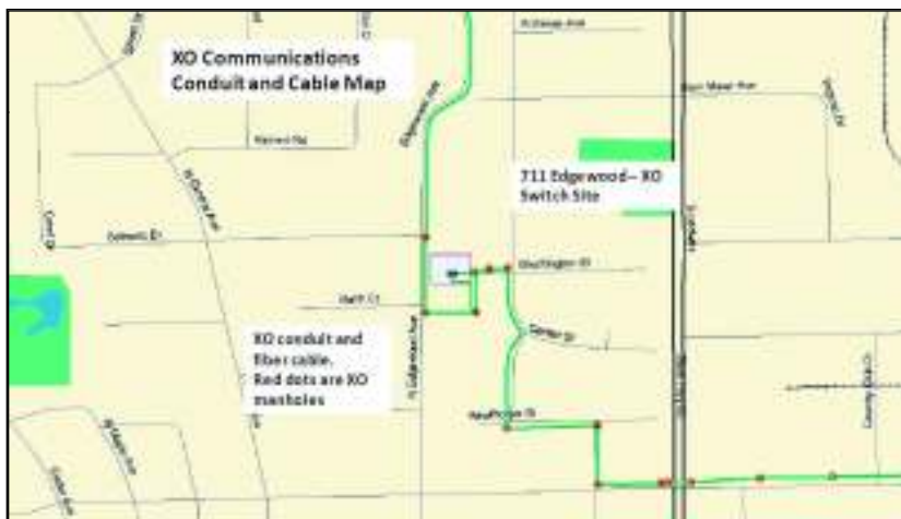
Figure 4.1: XO Communications Conduit and Cable Map
