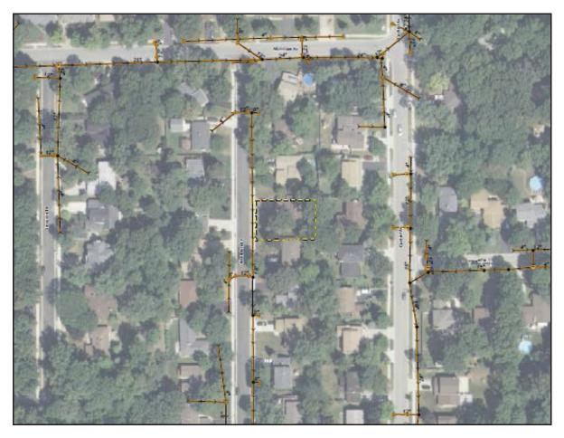
According to our existing conditions XP-SWMM model, the storm sewer system along Montclare Lane has excess capacity, but presently there is not a subsurface connection from the rear yard of the subject property to the sewer.
