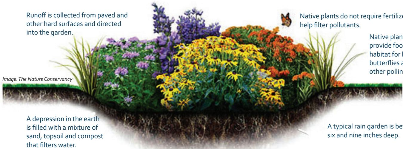
A depression in the earth is filled with a mixture of sand, topsoil and compost that filters water.
